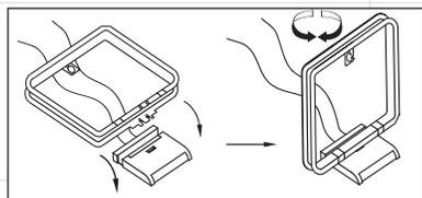
**1.** Assemble the supplied AM Loop Antenna as shown above. Connect it to the **AM** and **GND Terminals 22** on the back of the DCR600II.
