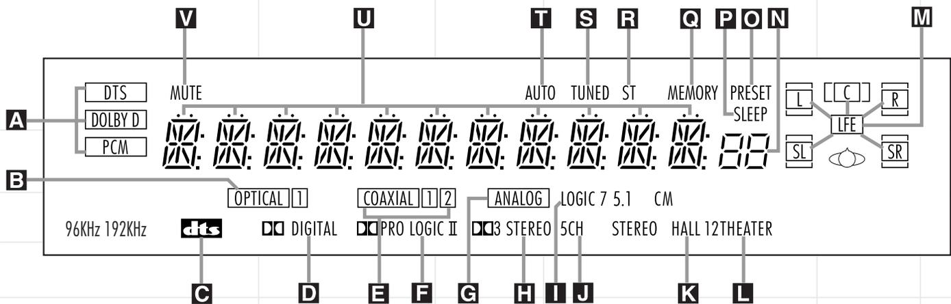
**A Bitstream Indicators:** When the input is a digital source, these indicators display the specific type of data signal. The DCR600II will also indicate when it detects a digital signal with a resolution of either 96kHz or 192kHz. This can occur when the receiver is used with an external DVD-Audio player or other device that is capable of transmitting this type of signal. You should not expect to see these indicators light when using the DVD600II as your source unit.
