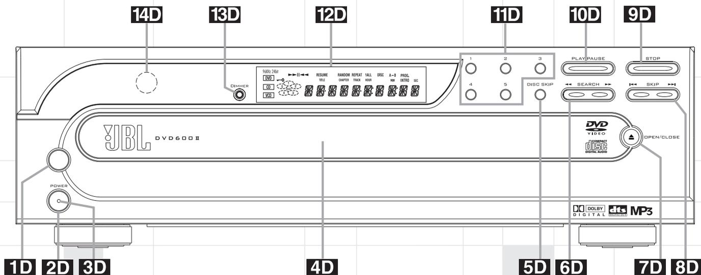
**1D Main Power Switch:** Press this button to apply power to the DVD600II. When the switch is pressed in, the unit is placed in a Standby mode, as indicated by the amber **Power Indicator 3D** surrounding the **System Power Control 2D**. This button MUST be pressed in to operate the unit. To turn the unit off and prevent the use of the remote control, this switch should be pressed until it pops out from the front panel so that the word "OFF" may be read at the top of the switch.
