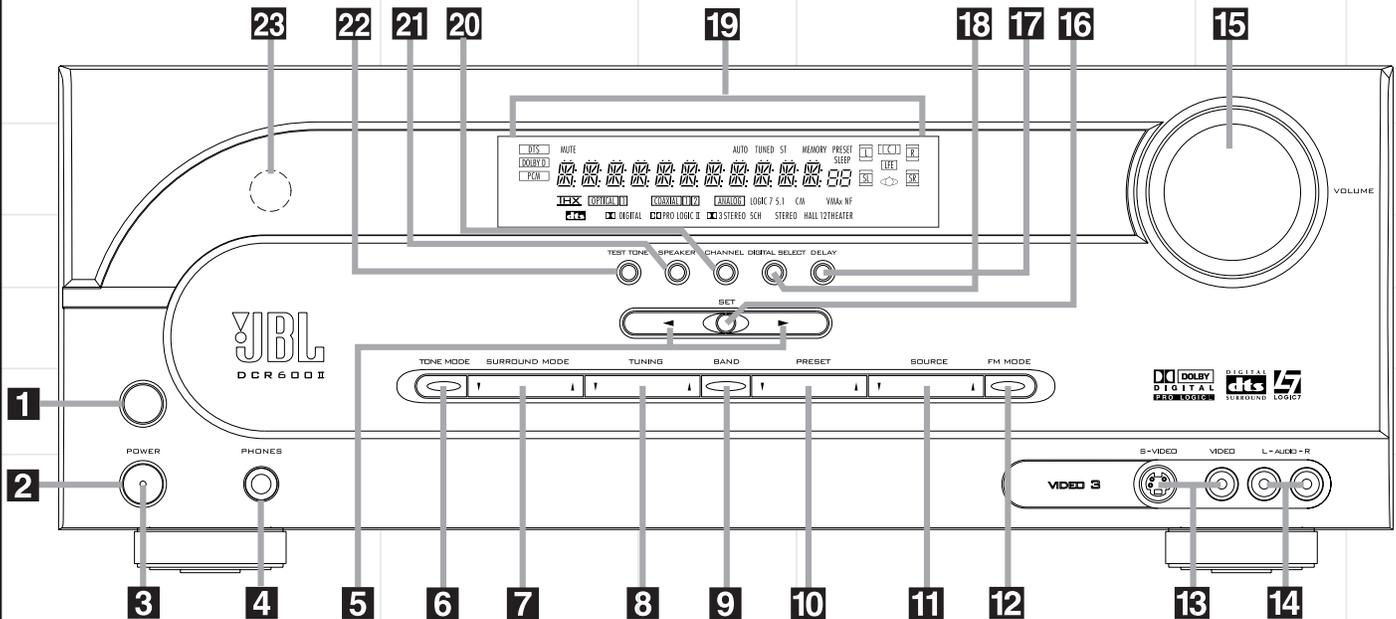
**1 Main Power Switch:** Press this button to apply power to the DCR600II. When the switch is pressed in, the unit is placed in a Standby mode, as indicated by the amber **Power Indicator 3** surrounding the **System Power Control 2**. This button **MUST** be pressed in to operate the unit. To turn the unit off and prevent the use of the remote control, this switch should be pressed until it pops out from the front panel so that the word "OFF" may be read at the top of the switch.
